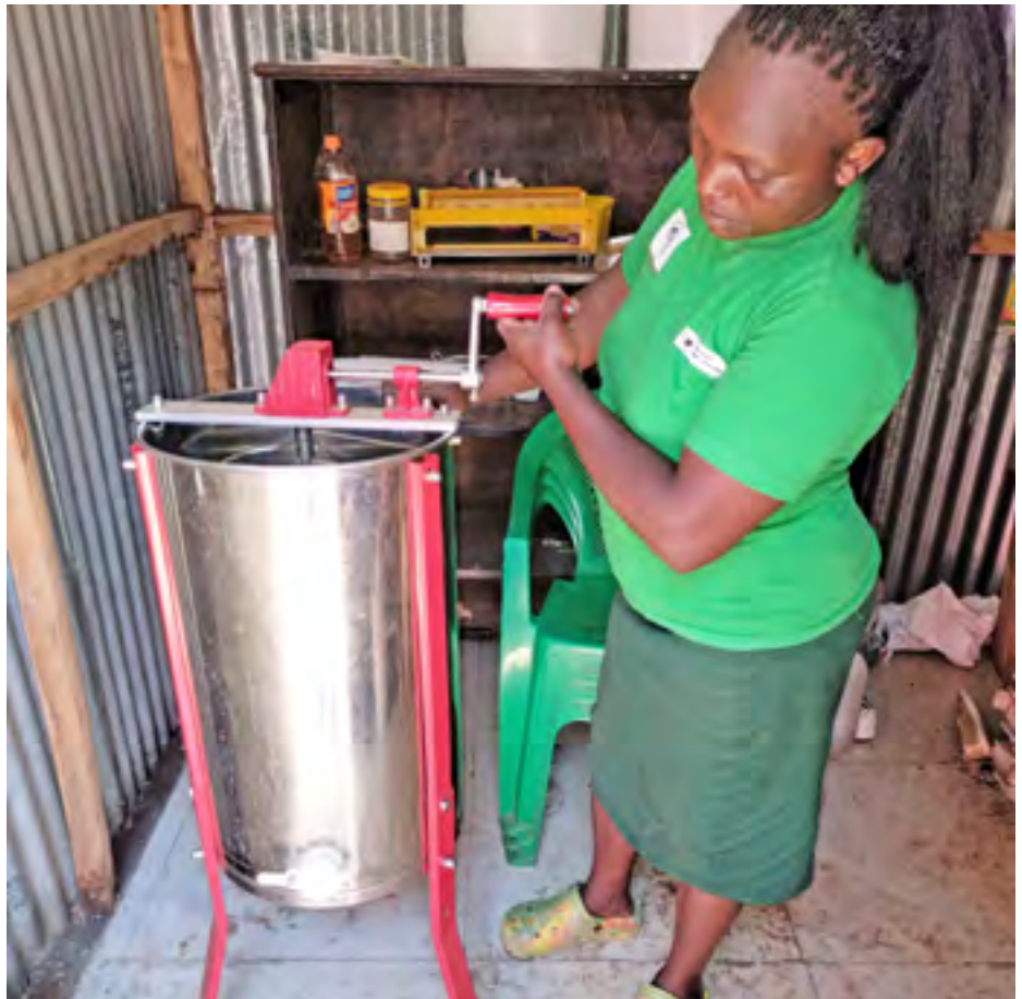
Mary Wanyoike demonstrates how a centrifugal honey processing machine works.
